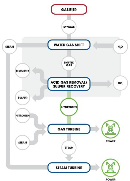
Converting the CO to  $CO_2$  prior to combustion is more economical than removing  $CO_2$  after combustion, effectively "de-carbonizing", or at least, reducing the carbon in the syngas.
