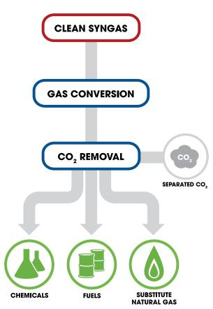
product at a time (co-production or "polygeneration"), such as the production of electricity, steam, and chemicals (e.g., methanol or ammonia). This polygeneration flexibility allows a facility to increase its efficiency and improve the economics of its operations.
